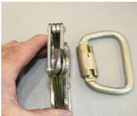
YOKE 263 Damaged Sleeve after Transition 10° Angle to Vertical Climb Test
