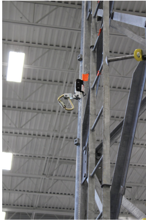
Shake Test Example - Safety Sleeve Un-Supported on the 7x19 Wire Rope
