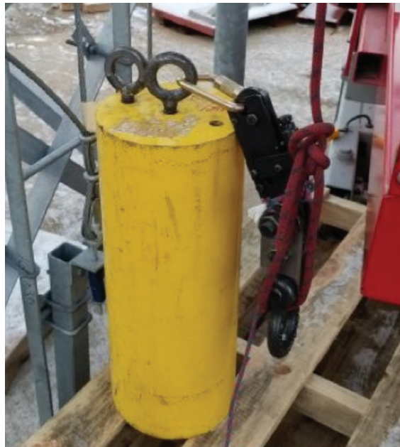
282 Pound Steel Test Cylinder with the Sweeney Quick Release Mechanism
