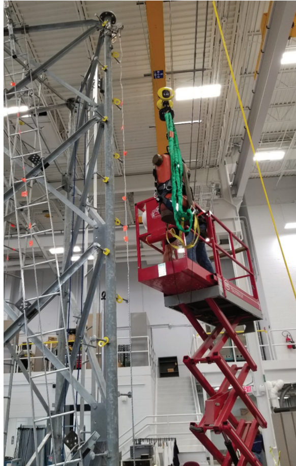
10° Lateral Climb Test - Ladder and Safety Climb System Set Up
