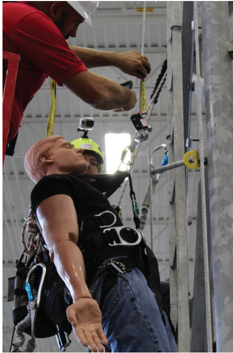
Sample Dynamic Test Drop with Weight ASling Safety Strap
