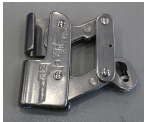
YOKE 263 Damaged Sleeve after Transition 10° Angle to Vertical Climb Test
