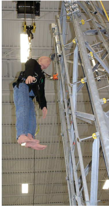
Dynamic Drop Test - Weight A - 1% Slack Test
