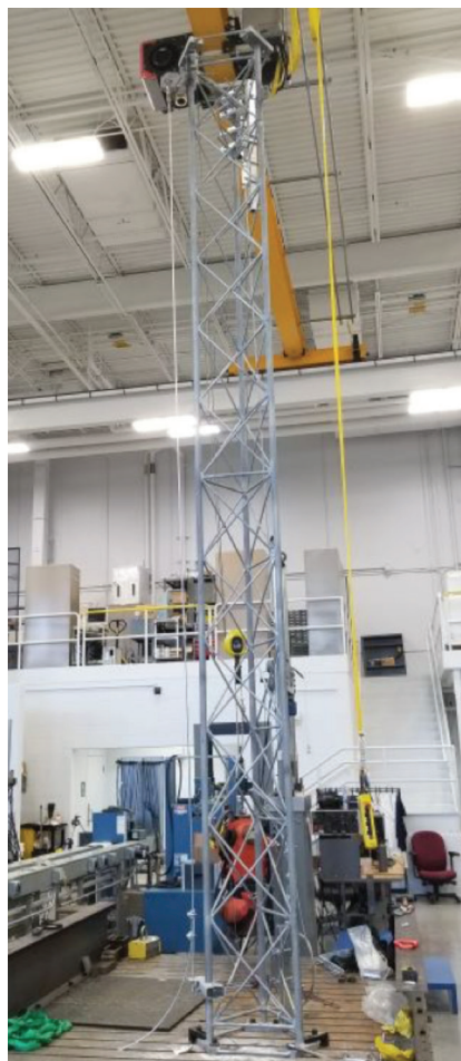
Test Tower Set Up for Part II Tests
