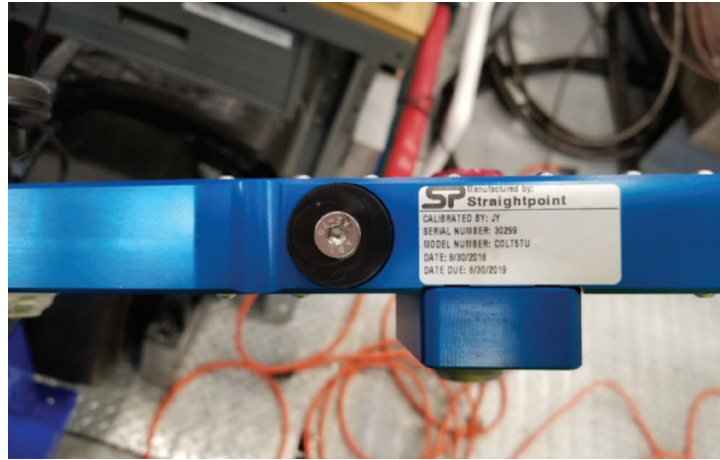
Straightpoint Tension Meter - Model COLT5TU - Serial Number 30299
