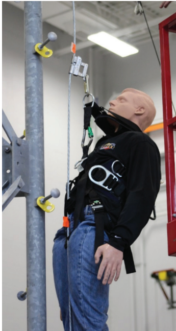
Test Weight A Dynamic Drop Test - 3M Safety Climb System 1x7 Wire Rope
