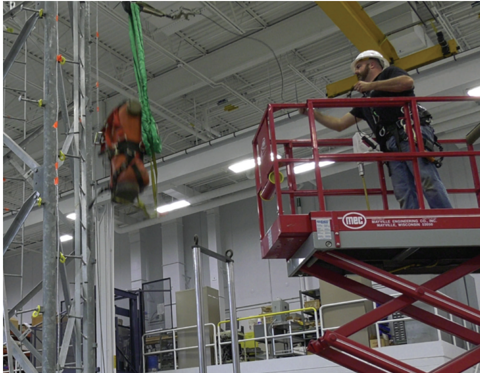
10° Lateral Climb Sample Test Drop in Motion
