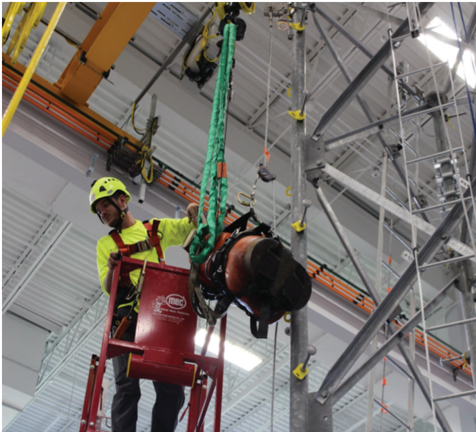
Dynamic Drop with 3M Lad Saf X3 Safety Sleeve and Test Weight B on 3M 1x7 Wire Rope Safety Climb System - Side Load on Carabineer After Drop
