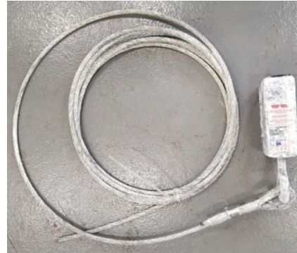
1x7 DBI Sala and 7x19 Tuf-Tug Wire Rope - 168 Hour Salt Spray
