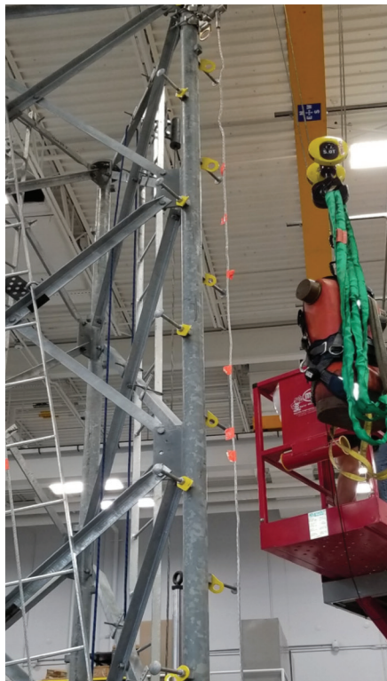
3M Safety Climb System with 1x7 Wire Rope Damage After 15 Drop Tests
