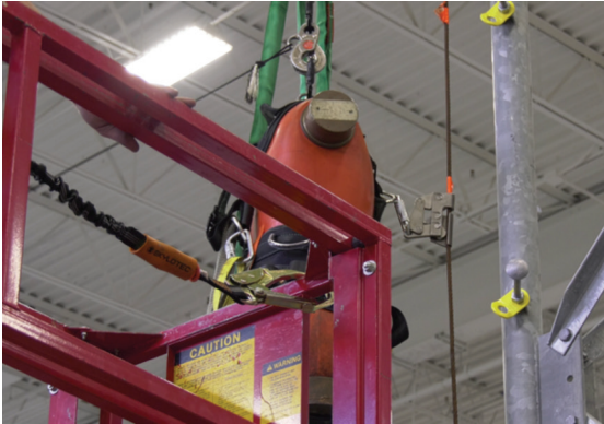
3/8" 7x19 Class 3 Corrosion Wire Rope Test
