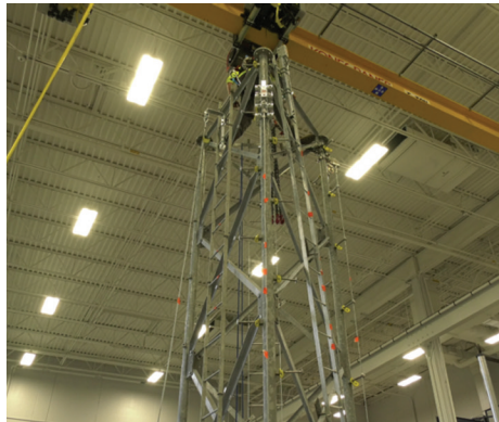
Trylon Safety Climb System - installed on the left side of the tower face after the 3rd Drop Test
