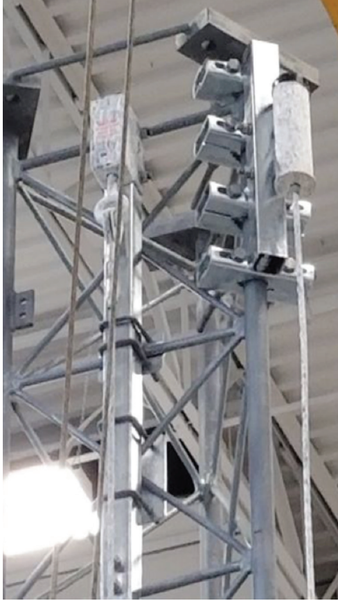
168 Hour Salt Spray Test - Tower Set Up
