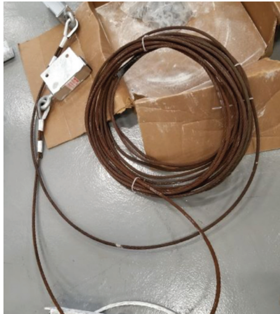
Corrosion Class 2 7x19 Wire Rope Safety Climb
