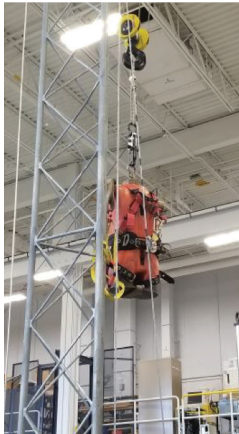
Transition 10° Angle to Vertical Test - Ready for Drop
