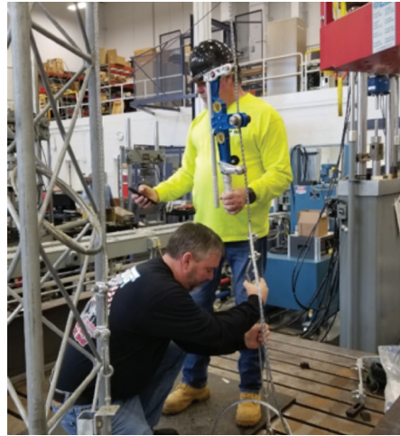
Tension Check Between Test Drops
