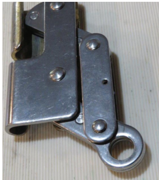
Used CABLOC PROTECTA 3/8" Safety Sleeve for 7x19 Wire Rope Only
