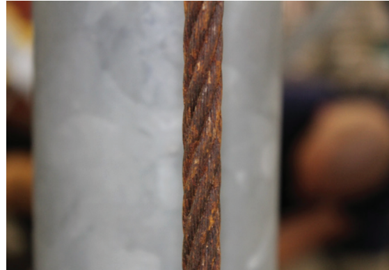
3/8" 7x19 Class 3 Corrosion Wire Rope Test
