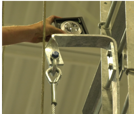
Trylon Safety Climb System after 3rd Test Weight B Drop Test
