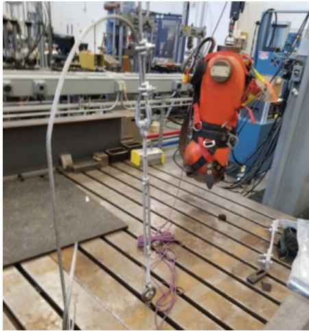
Transition 10° Angle to Vertical Test Base Assembly Set Up
