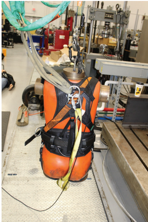
Test Weight B with Sling Safety Strap
