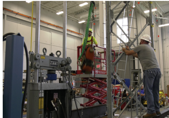
Transition 10° Angle to Vertical Climb Test - Set Up and Release of Test Weight B
