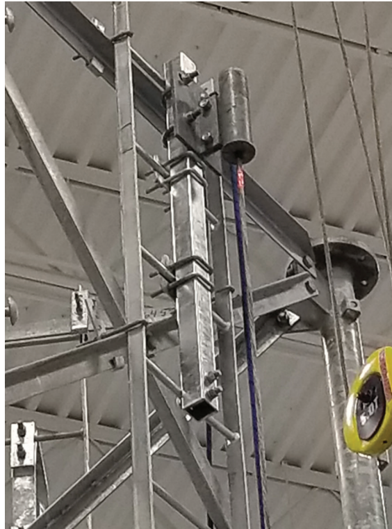
Used DBI SALA 1x7 Wire Rope Safety Climb - Bird Dropping Wire Rope Test
