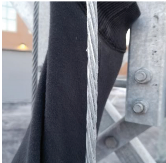
Thin Film Ice on the Wire Rope
