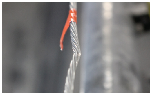
3/8" 1x7 Galvanized 3M System Wire Rope Damage from Test Weight B Drop
